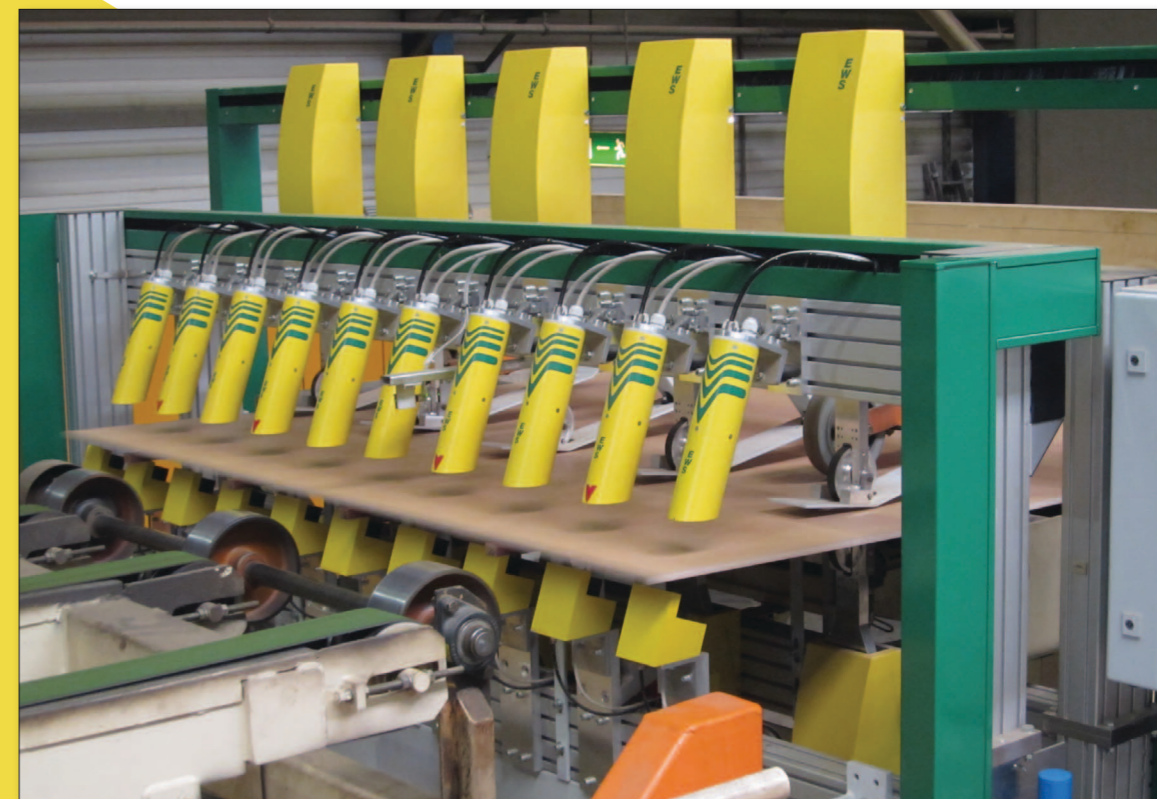
EWS blow detection and thickness gauge system installed on a panel line
