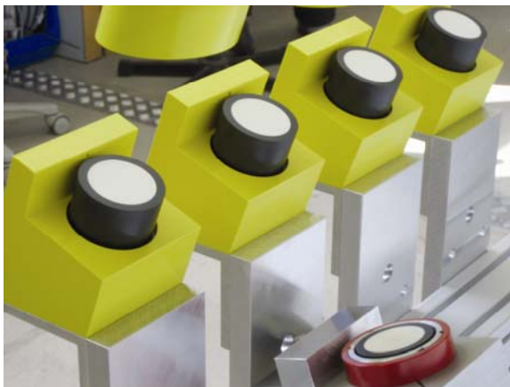
CONTI-SOUND Early Warning System equipped with additional reflection receivers (red)
